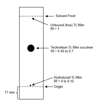
Rf =  $\frac{\text{Distance (from origin) travelled by solute (Tc 99m compound)}}{\text{Distance (from origin) travelled by solvent (n-butanol /3N HCl)}}$
